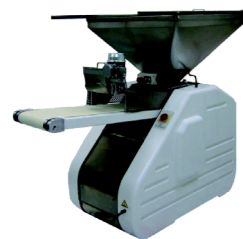
Division Volume divider: open hopper - closed manual or automatic hopper
