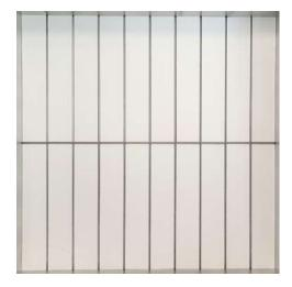
In its **Double Cut** version, DiviTrad Compact divides your dough directly into 2x10 pieces. Cutting during the tamping phase produces dough pieces that are less degassed, well sealed and gently elongated, to preserve the dough and guarantee future honeycombing.
