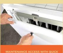
MAINTENANCE ACCESS WITH QUICK ACCESS RELEASE SYSTEM FOR EASY DAILY CLEANING OF THE MACHINE INTERIOR.
