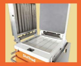
With its 400x400 mm bowl, DiviTrad® Compact is equipped with knives for cutting into 20 square dough pieces. It allows both "classic" division before proofing and "traditional" division to form baguettes and bake immediately.
